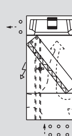
▶ Down Suction / Front Flow
